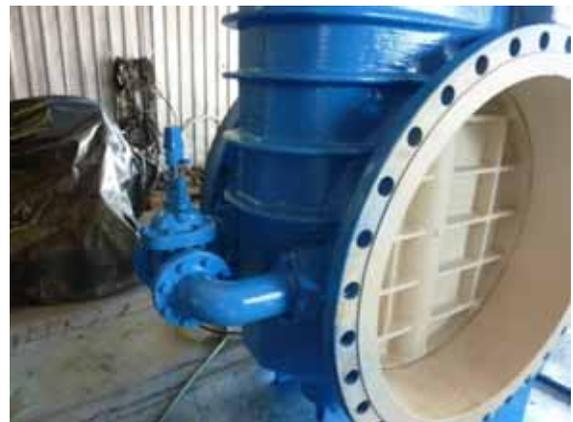
Figure 2: Seat test at Premier Valve factory
